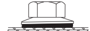
TOO LOOSE Sealant is not compressed and can not form a seal.
